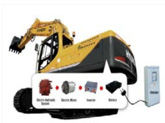
• 21-ton Battery-powered Excavator
